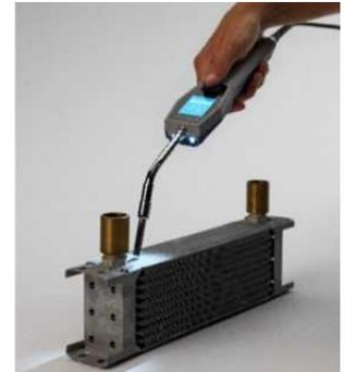
**Leak testing soldered oil cooler connections**
